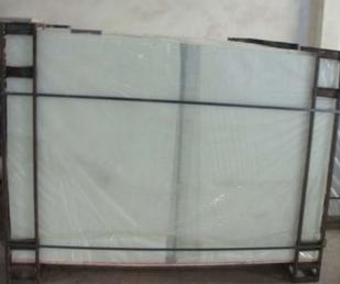
Whatever the size is, a standard binding will be taken where just in need. Professional loading and fixxing plus our advanced steel end-cap offer us safely and high efficiency solution. We great succeed deliver thousand containers glass without any breakage duce to our pakage.
