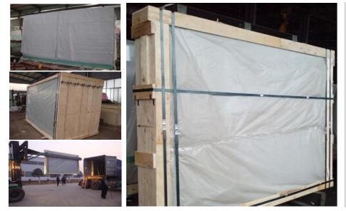
Whatever the size is, a standard binding will be taken where just in need. Professional loading and fixxing plus our advanced steel endcap offer us safely and high efficiency solution. We great succeed deliver thousand containers glass without any breakage.
